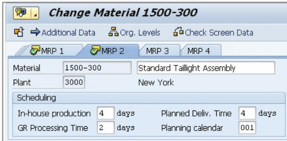
Figure 4 Planning Calendar Entered into Material Master Record
