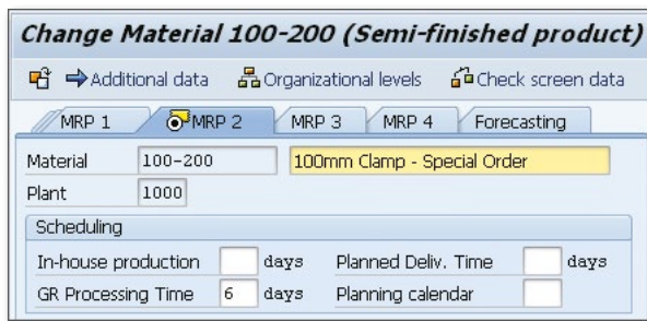
Figure 1 Goods Receipt Processing Time Shown in the Material Master Record
